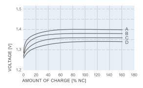
Charging curves at various charging currents of NiMH Button Cells V...H(T) at 0°C
