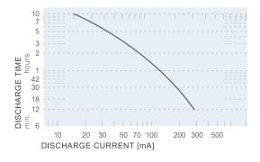
FIG. 6 Discharge curves of V7/8H
