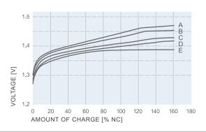
FIG. 27 Charging curves at various charging currents of NiMH Button Cells V...H(T) at +45°C
