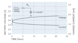
Trickle charge characteristics of e.g. 2/V 18 HRT  $R_C$  = 1  $k\Omega$
