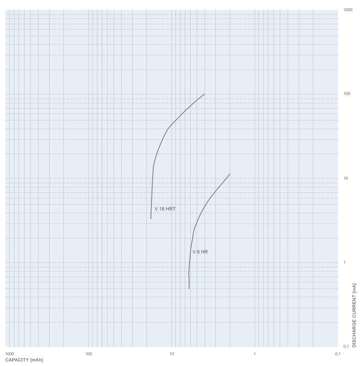
FIG. 36 Discharge characteristics V 18 HRT, V 6 HR
