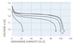
Relative capacities, based on the effective capacity (= 100 % C at room temperature) as a function of the discharge temperature at 0.2 CA
