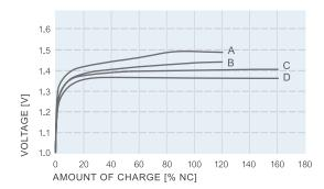
Charging curves at various charging currents of NiMH High Rate Button Cells V...HR at 0°C
