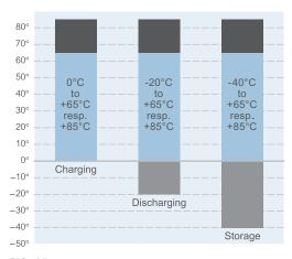
Permissible temperature range for NiMH High Rate Button Cells (+65°C resp. +85°C, depending on type. See also p. 27)
