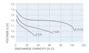
Typical discharge curves of NiMH Button Cells at +23°C
