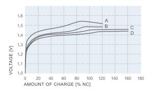
FIG. 30 Charging curves at various charging currents of NiMH High Rate Button Cells V...HR at +45°C
