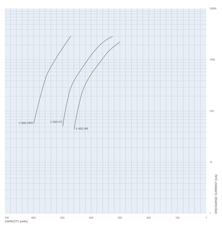
FIG. 35 Discharge characteristics V 600 HRT, V 500 HT, V 450 HR
