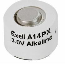
Industry Standard Dimensions mm (inches) Chemical System:AlkalineDesignation:ANSI/NEDA-1201MP,IEC-2MR9Battery Voltage:3 VoltsAverage Weight:11.3 grams (0.4 oz.)Volume:3.4 cubic centimeters (0.2 cubic inch)Average Capacity:178 mAh to 0.8 volts/cell<br/>(Rated at 25 mA continuous drain at 21°C)Jacket:Cardboard
