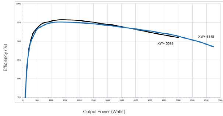
Figure 19.0 - Conext WX+ Efficiency vs Load Graph
