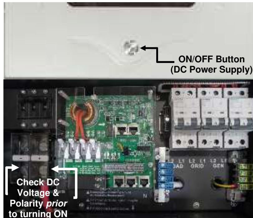
Figure 18.0 – Inverter & DC Power Supply ON/OFF Button
